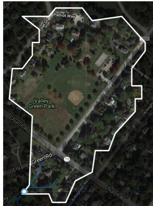
The park receives some water from Patriot Way and Redcoat Drive, but most of the stormwater is generated in the park.
