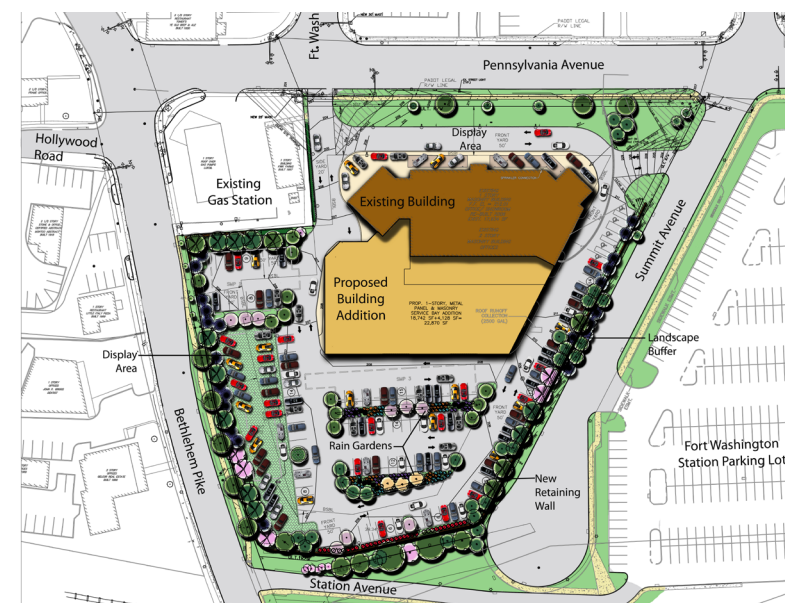
Mercedes of Fort Washington submitted Land Development Plans to the Township in June of 2010 to add a service facility on-site. The plan proposes an increase in building coverage from the existing 14.2% to 26.2%, but proposes a decrease in impervious coverage from the existing 85.6% to 75.3% with an increase in green area from the existing 14.4% to 24.7%.
