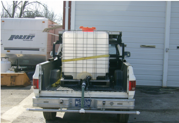
Above, industrial sized brind system. Below, township's in-house made brind system.
