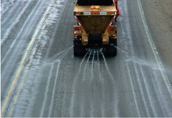
Above, industrial sized brind system. Below, township's in-house made brind system.
